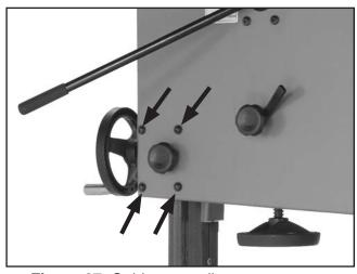
Figure 67. Guide post adjustment screws.
